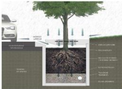
TREE-LINED FILTER BOXES
