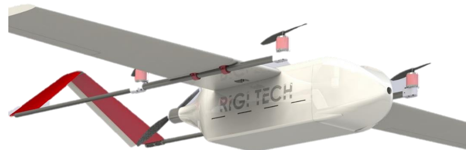
Octacopter ID8HSE (10 kg payload)
